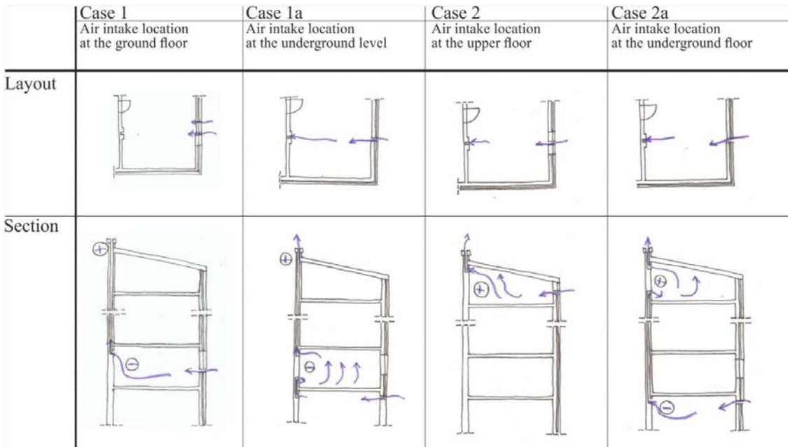
Figure 2: Study on the natural balanced ventilation system. Assessment of the air pressure, draught in the ventilation system with regard to the changing air intake location. Author: Student G. Konieczny. Supervisor: T. Gaczoł (Source: Archive of the Chair of Building Design, Faculty of Architecture at Cracow University of Technology).
